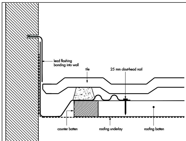
*Figure 2 Filon GRP Abutment Secret Gutter/Soaker (GAS 1) with slate roof application*
