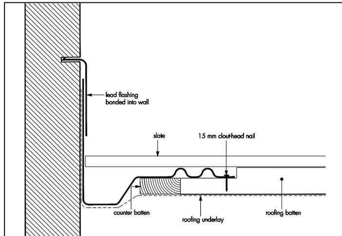
1.2 The profile is supplied in lengths of 3 m, with a width of 140 mm.
