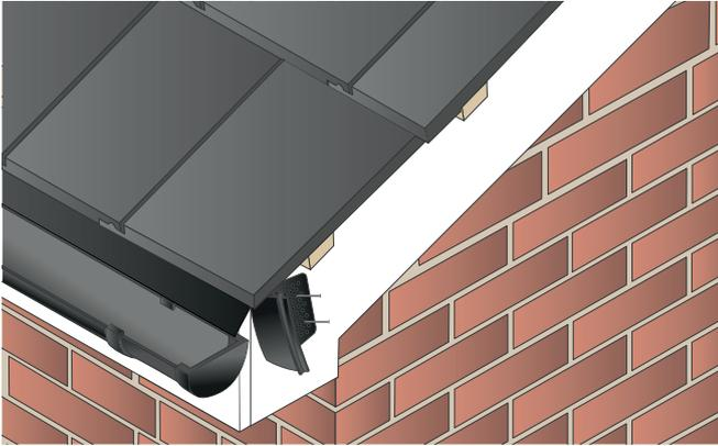
3 Snap the starter kit off the blanking plate. Starting at the bottom edge of the roof, insert the starter piece into the front end of the verge unit, and mark out the starter piece position on the fascia and barge board. Remove the unit and mechanically fix the starter piece into position through the grid.
