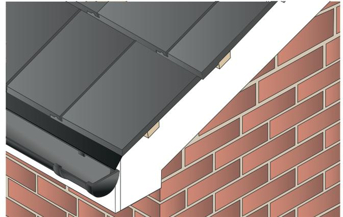
**2** Lay tiles set flush with the battens. Remove existing mortar bedding in refurbishment project and install new tiling batten to the underside of the existing tiling batten.
