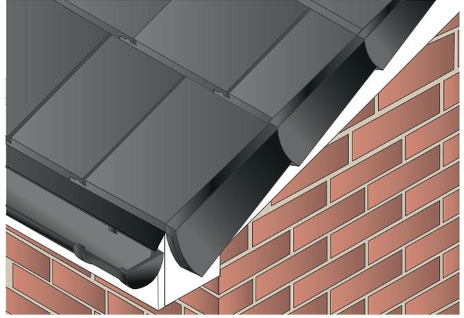
6 Continue the process up along the barge board, until the ridge. If required, insert the blanking plate over the final verge nail grid to prevent water ingress. Now insert the ridge cap once the other verge is completed.
